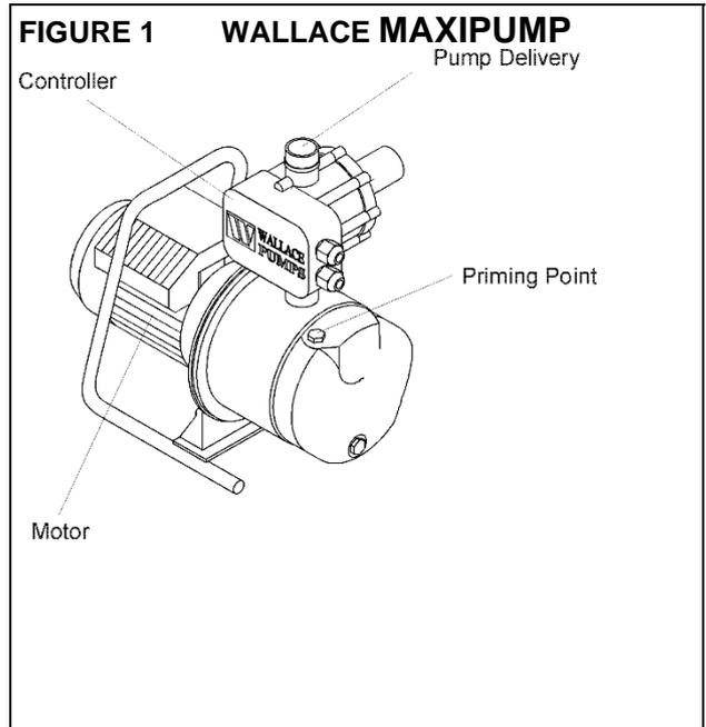
**Filters:** Do not install any other filter in the pipework between the water source and pump. Only install filters on the pump delivery, be aware that filters can reduce pump delivery flow and pressure, and need frequent servicing.
